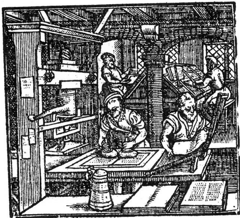
A sixteenth-century printing shop. From Stephen Batman, The Doom Warning All Men to the Judgment (1581). The printing press here shown, in all essentials typical of presses used down to the end of the eighteenth century, is being worked at "full press" (i.e. with two men), one man (right) removing from the tympan a sheet just printed off, the other inking the type-bed with the ink-balls, preparatory to the next "pull." Note (left) the "platen" (half the size of a sheet), fastened flexibly at the lower end of the large screw spindle, which, when the carriage was slid back under it, was brought down evenly and firmly on the type-bed by a strong pull of the "bar" to make the impression. In the foreground are two "piles," one of sheets already printed off in the press-run, the other of sheets still waiting to be "impressed." In the rear of the shop a compositor (right), sitting before a "case" of type, is seen setting from "copy," which is held in a copy-holder to his left. Opposite him, another compositor is either making press-corrections or setting type. (By permission of the Harvard College Library)
